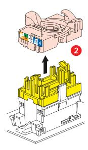
This system allows the wire pairs to be spread easily before attaching them to the connector.
