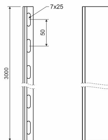
**product description:** The partition is used to separate cables in cable trays. In term of electrical compatibility, it is also used for dividing several types of lines. It is recommended to use covers for this type of installation and make the covered and shielded room.
