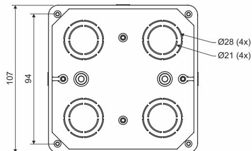
product description: designed for distribution system with voltage 400 V and with maximum current 16 A
