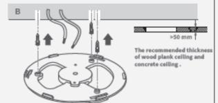
Applied for the ceiling installation of light weight ceiling, wood plank ceiling, or concrete ceiling. (4) According to the requirements of the following scheme, it is necessary to remove isolation from the wire on 8-9mm.
