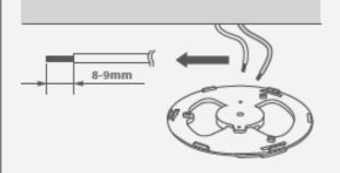
(5) Press the pink button and insert a cord into the terminal block, then make sure the reliability of connection.
