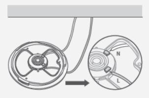
(6) Hold the lamp body to align and fix in the base. Rotate the lamp body to the left and right to remove and install.
