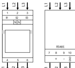
RS-485 cable recommended: shielded and twisted pair, 2 x 0,5 mm<sup>2</sup>.
