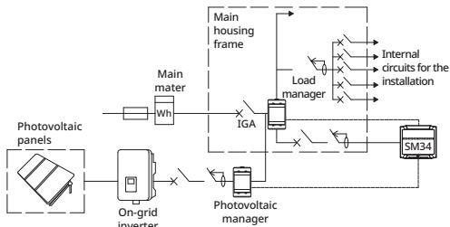
**Warning!** Verify that the load manager (0695000-400) measures all household consumption, including consumption by the electric vehicle. The photovoltaic manager should only measure photovoltaic generation.
