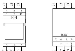
RS-485 cable recommended: shielded and twisted pair, 2 x 0,5 mm<sup>2</sup>.
